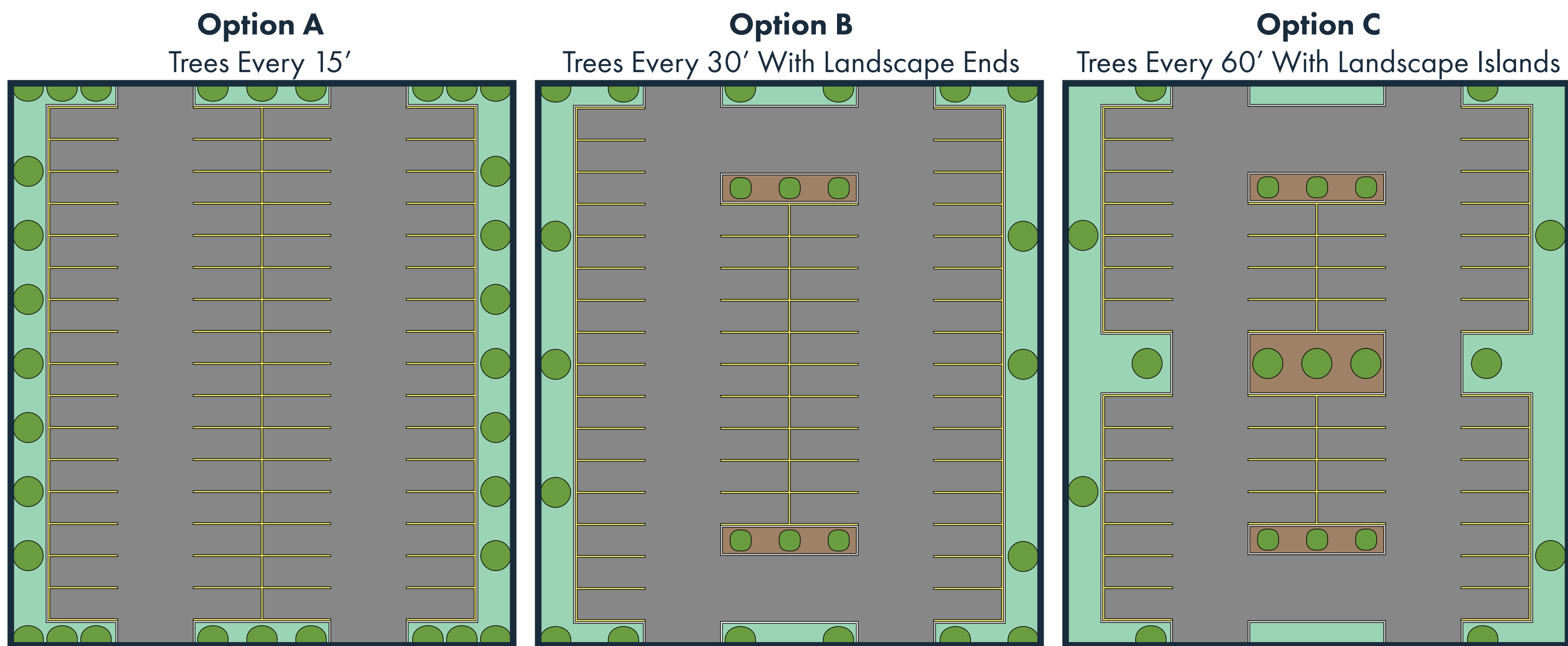
Example of possible parking lot screening requirements
