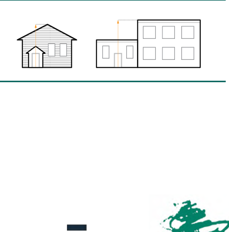
Exhibit 6-3. Measuring principal building height
